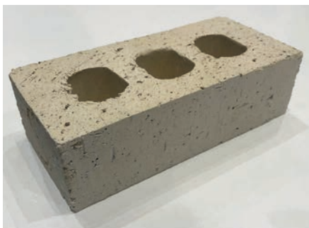
A brick made from DBS sand. One of many potential applications that are currently being studied. (Image: ILiA)
