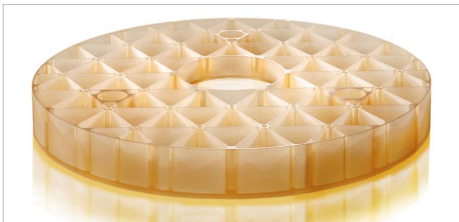
ZERODUR® mirror substrates for space optics are lightened using precision grinding to remove up to 90% of the original casting, while maintaining the strength needed to survive the launch and in harsh space environments. (Image: SCHOTT)
