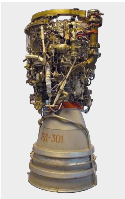
Bilderling RD-301 Rocket Engine.
