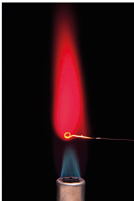
Lithium ions react in the flame of a Bunsen burner. Lithium is unusual as it reacts with both the oxygen to form lithium oxide ( \text{Li}_2\text{O} ) and nitrogen to form lithium nitride ( \text{Li}_3\text{N} ).
